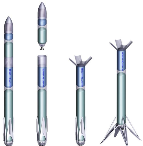
Conceptual sketch of the RETALT1 spacecraft. Configurations from left to right: launch, stage separation, first stage descent, first stage landing.
